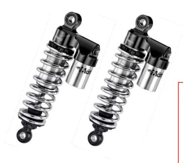
Two-way adjustable hydraulic shock with separate pressurized expansion tank (Nitrogen gas N<sub>2</sub>). Shock and tank cylinder d.40 mm in Aluminium alloy (Al 7075) with lapping and oxidation surface treatment. Piston rod d.16 mm in high tensile alloy steel with hard Chrome surface coating. Damper adjustment by two distinct and indipendent adj. units:
