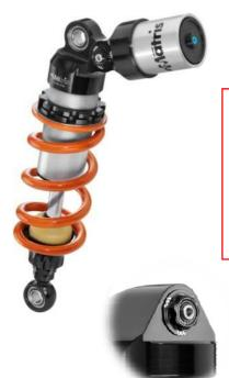
Two-way adjustable hydraulic monoshock with separate pressurized expansion tank (Nitrogen gas N<sub>2</sub>).
